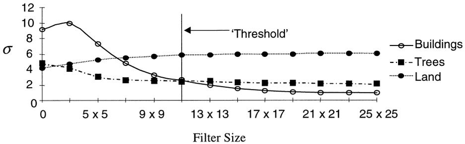
Fig. 5. The effects on standard deviation ( $\sigma$ ) with respect to filter sizes for different feature types.
