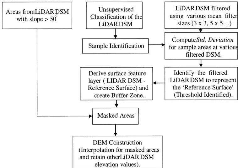
Fig. 7. Outline methodology for constructing the Digital Elevation Model (DEM) from the LiDAR Digital Surface Model (DSM).
