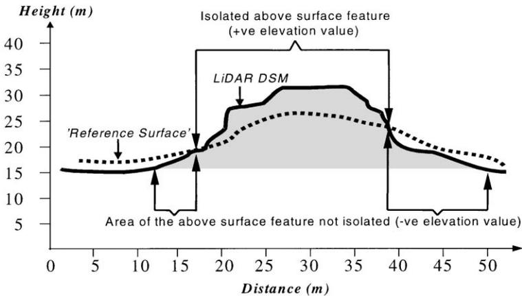
Fig. 6. The effect of subtracting the ‘reference surface’ from the LiDAR Digital Surface Model (DSM).
