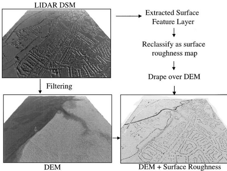
Fig. 8. The separation of the Digital Elevation Model (DEM) and surface roughness.
