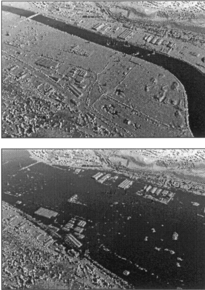
Fig. 2. A simple river flooding simulation using a LiDAR Digital Surface Model (DSM).
