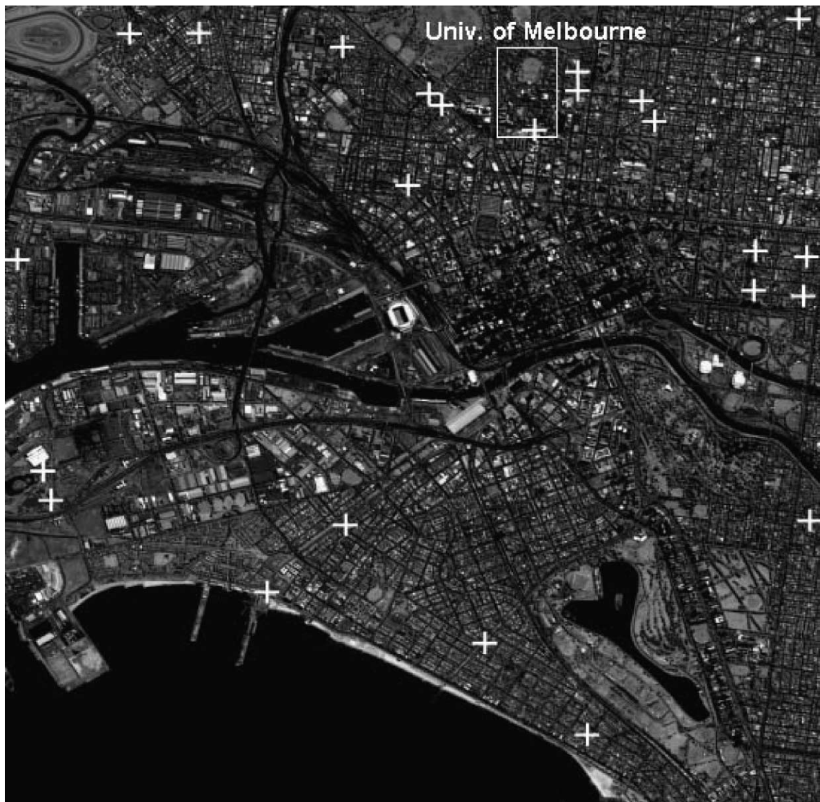
Fig. 1. Ikonos Geo panchromatic nadir image of Melbourne showing the distribution of control points and the University of Melbourne campus.
