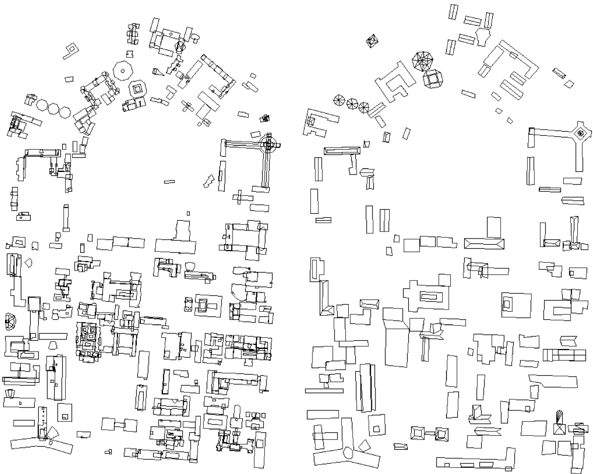
Fig. 7. Buildings of University of Melbourne campus reconstructed from 1:15,000 aerial images (left) and stereo Ikonos imagery (right). To simplify visualisation, first points and first lines have been omitted in the left figure.
